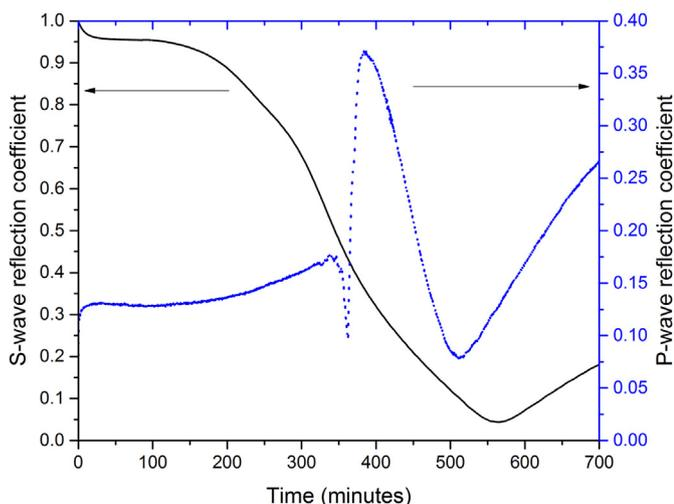
Fig. 1. Typical P-wave and S-wave UWR responses of ordinary type I cement paste with w/c 0.5.
