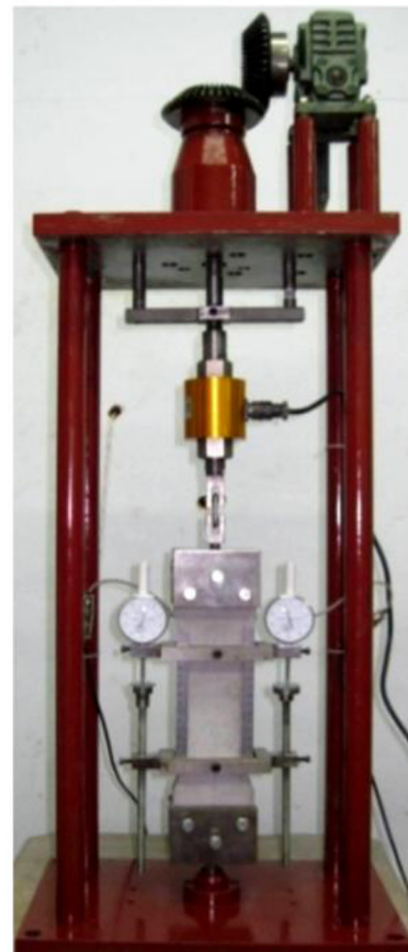
Fig. 2. Direct tension test imposed on the specimens to create multiple cracks under different levels of tensile strain.
