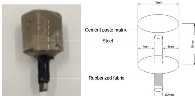
Fig. 1. Schematic presentation of specimens.
