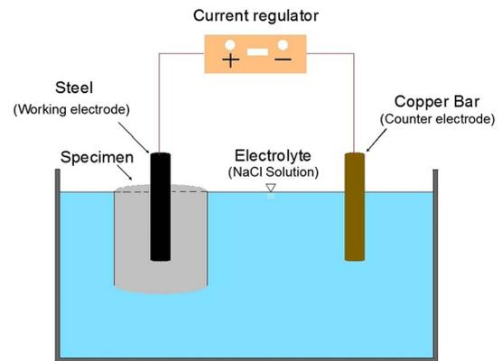
Fig. 2. Schematic illustration of accelerated corrosion procedure.
