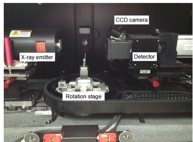
Fig. 3. Internal features of XRadia Micro XCT-400.
