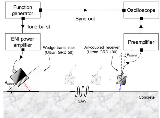
Fig. 1. Schematic of the SHG setup.
