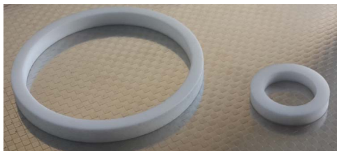
Fig. 1. PTFE rings used as a deformable die. Smaller diameter ring on the right was used for preliminary experiments. While the one on the left was used to fabricate 2 in. diameter \text{La}_{0.8}\text{Sr}_{0.2}\text{CoO}_{3-\delta} (LSC-113) sputter target.
