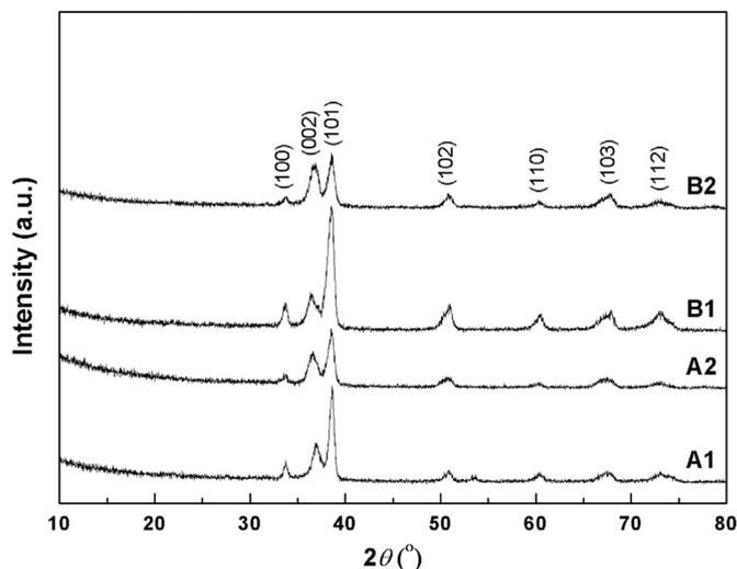
Fig. 1. XRD patterns of the vitroceraic coatings deposited by PLD from A and B targets, on Ti-Zr substrates.
