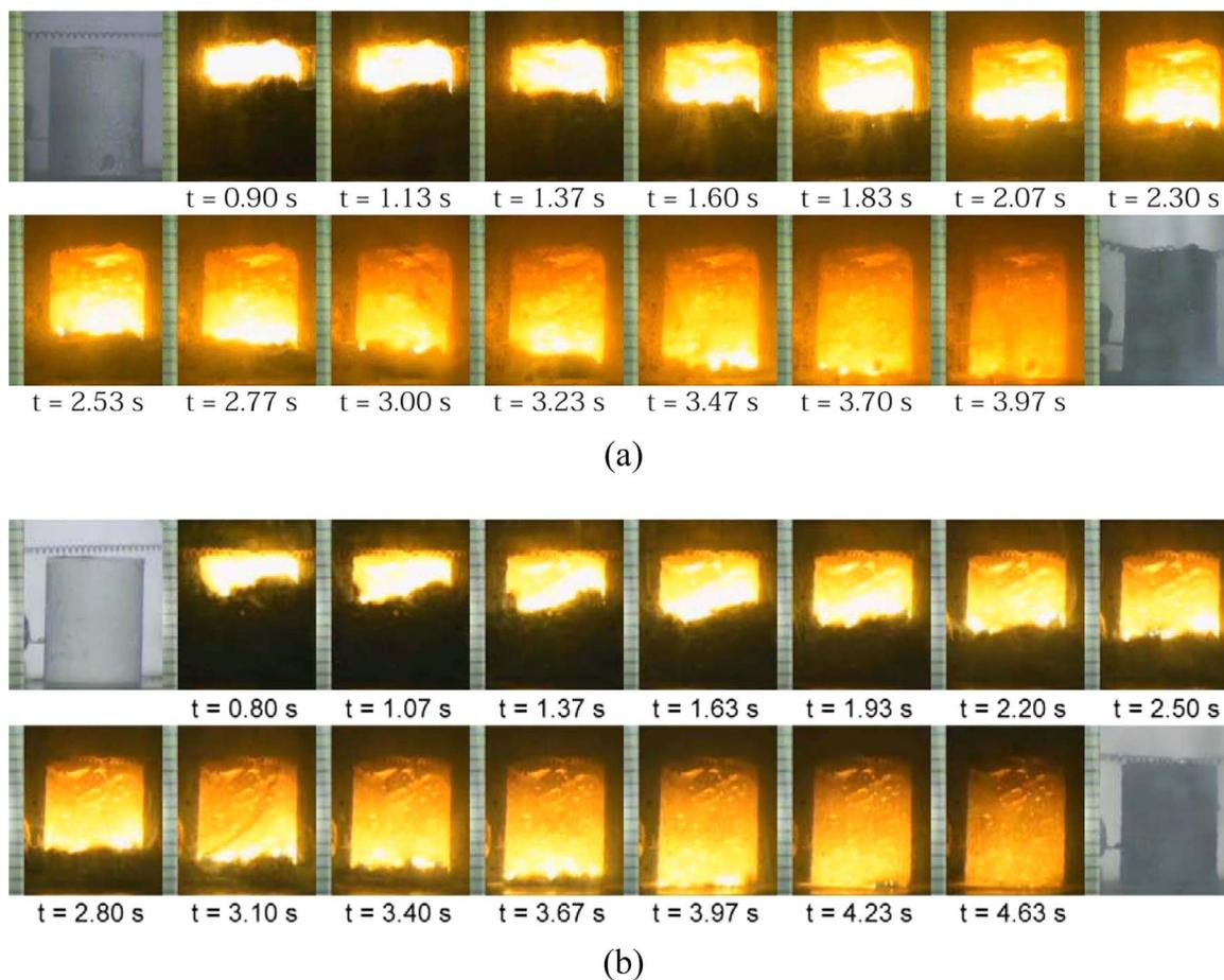
**Fig. 1.** Time sequences of recorded images illustrating self-sustaining combustion wave propagating along samples of (a) Reaction (1) with  $y/x=1.25$  and (b) Reaction (2) with  $n/m=2.0$ .
