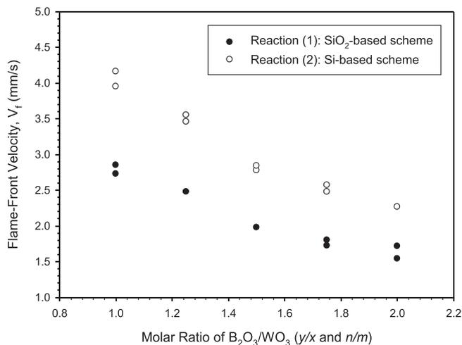
**Fig. 2.** Effects of molar ratio of  $\text{B}_2\text{O}_3/\text{WO}_3$  on flame-front velocity of  $\text{SiO}_2$ - and Si-based reaction systems.
