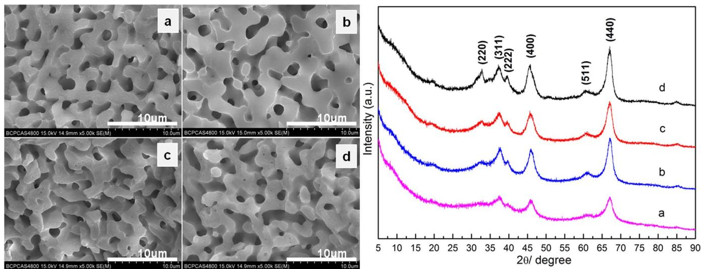
Fig. 2. SEM and XRD patterns of alumina calcined at 973 K (a), 1073 K (b), 1173 K (c), 1273 K (d).
