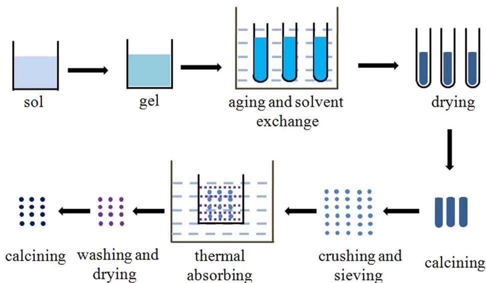
Fig. 1. Schematic illustration of the synthetic process of  $\text{Al}_2\text{O}_3$  monoliths.
