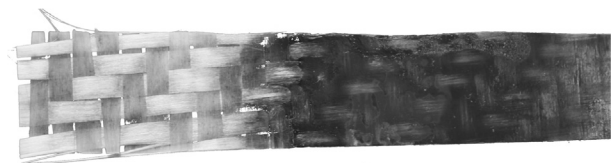
Fig. 2. Tepex material; matrix removed on left side, exposing the glass weave. (For interpretation of the references to colour in this figure legend, the reader is referred to the web version of this article.)
