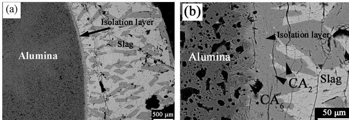
**Fig. 1.** SEM images of the reaction interface between slag S1 and alumina A1.
