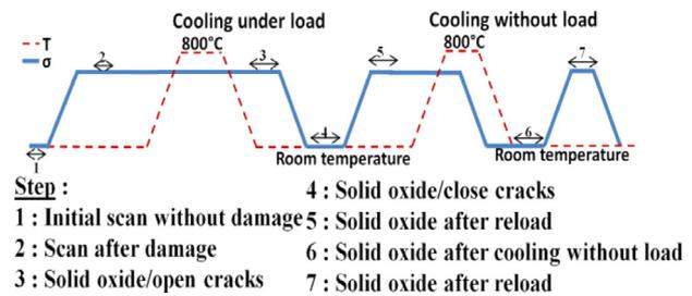
**Fig. 2.** Schematic description of in situ tension tests performed at high temperature in  $\mu$ CT.
