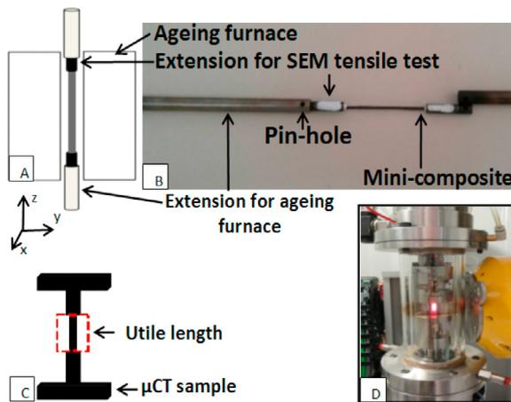
**Fig. 1.** (A) Schematic representation of the ageing furnace, (B) extension for the ageing furnace and the SEM tensile test, (C)  $\mu$ CT sample, (D) picture of the tension device in the GE/VTomx  $\mu$ CT with a specimen heated at 1000 °C.
