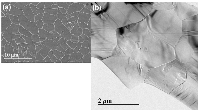
Fig. 2. Typical microstructure of SiC ceramic sintered with 2000 ppm  $Y_2O_3$ : (a) SEM and (b) TEM images. The SiC ceramic consists of slightly elongated grains and liquid pockets at the triple junctions. Liquid pockets are not frequently observed.
