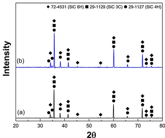
Fig. 1. X-ray diffraction patterns: (a) as-sintered SiC ceramic with 2000 ppm  $Y_2O_3$  and (b) SiC ceramic tested at 2000 °C.
