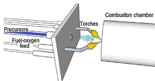
Fig. 1. Flame spray pyrolysis equipment.
