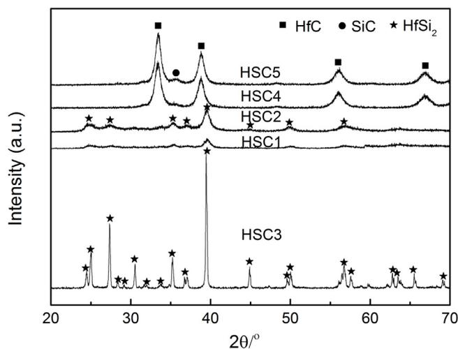
Fig. 1. XRD patterns of the different starting powders after mixing.
