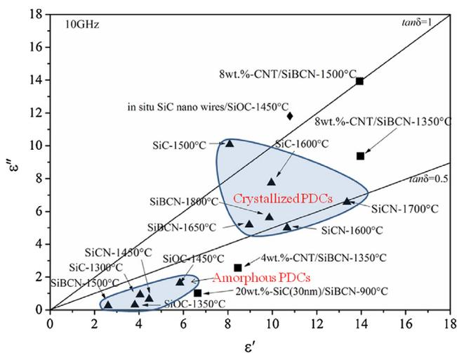
Fig. 1. Some reported dielectric properties of PDCs-SiC [11], SiCN [12], SiOC [14], SiBCN [16], SiC/SiBCN [17] and CNT/SiBCN [18].
