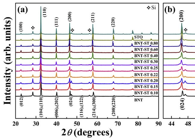
Fig. 1. XRD patterns of BNT-STx bulk ceramics with selected angles of (a) 20–90° and (b) 43–49°. (Note: Si powder was used as a standard for X-ray diffraction and the XRD peaks are indexed with rhombohedral (bottom) and cubic (top) structure.)
