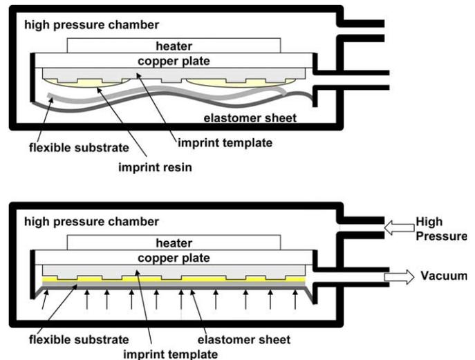
Fig. 2. Schematic diagram of an imprinting system. For the delivery of uniform pressing force over large area substrate, imprinting system is based on pressurized chamber.
