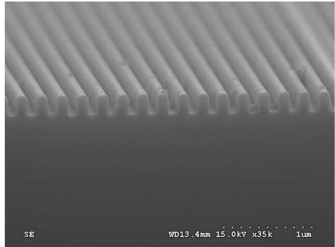
Fig. 1. Cross-sectional SEM micrograph of Si template, which has the dense array of 100 nm lines and spaces.
