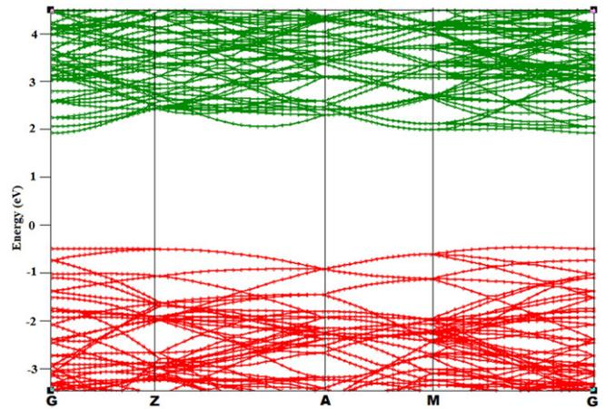
Fig. 2. Band structure of  $\text{TiO}_2$  nanostructures [G - gamma point-Center of Brillouin Zone (0, 0, 0), Z - Center of a square face (0, 0, 0.5), A - Corner point in simple tetragonal (0.5, 0.5, 0.5), M - Center of an edge (0.5, 0.5, 0)].
