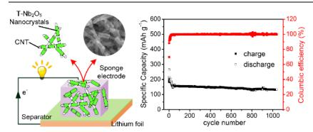
T-Nb<sub>2</sub>O<sub>5</sub> nanocrystals are *in situ* grown in CNT sponges and serve as binder-free, safe and stable lithium ion battery anodes.
