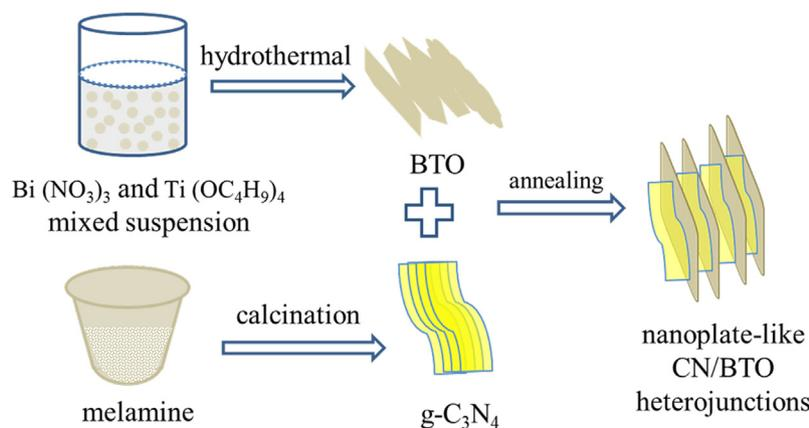
**Scheme 1.** Schematic illustration for the synthetic procedure of CN/BTO heterojunctions.
