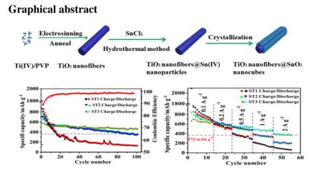
Hierarchically heterostructured  $TiO_2@SnO_2$  core-branch nanofibers are synthesized with promising electrochemical performance as anodes for lithium-ion batteries.
