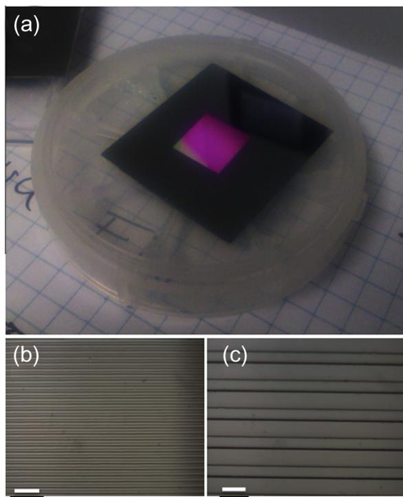
**Fig. 1.** Substrates. (a) Representative images of the micropatterned molds. The structure was created by electron beam lithography on a thin layer of SU8 resist. The patterned area is 1  $\text{cm}^2$ . (b, c) Representative images of T4 and T20 PDMS membranes acquired by bright field optical microscopy. Samples were fabricated by replica molding. Scale bar = 16  $\mu\text{m}$ .
