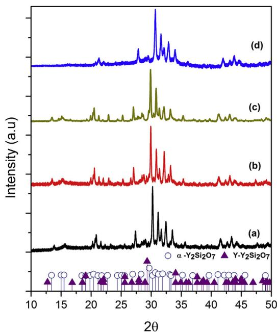
Fig. 1. XRD patterns of the (a) 1% per mole (b) 2% per mole and (c) 5% per mole  $\text{Yb}^{3+}$  doped and (d) undoped  $\text{Y}_2\text{Si}_2\text{O}_7$  nanoposphors annealed at  $1250^\circ\text{C}$  for 12 h.
