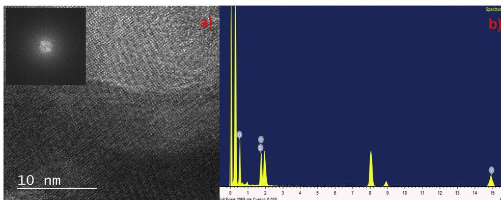
Fig. 2. a) Transmission Electron Microscopy (TEM) b) Energy-dispersive X-ray spectroscopy (EDS) images of undoped yttrium silicate powder.
