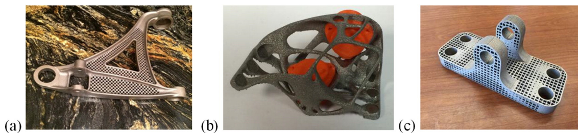
Fig. 2. Load-bearing structural components that are fabricated by additive manufacturing. (a) An automotive control arm printed by the binder jetting process in 420 stainless steel (courtesy of Jeff Shepler (ExOne)), (b) An accelerometer bracket printed by the electron beam method (EBM) in titanium alloy (courtesy of Keith Roberts (AMRDEC) and Devlin Hayduke (Materials Sciences Corporation)), and (c) A lattice structured pillow bracket fabricated by the selective laser melting process in titanium alloy.
