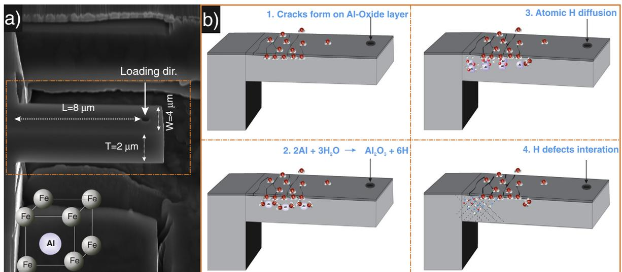
Fig. 1. Side view of a FIB-milled FeAl single crystal cantilever before bending a); the principle of in-situ hydrogen charging within ESEM mode b).
