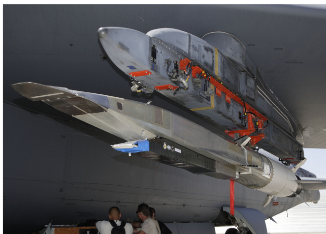
Fig. 2. Photograph of the X-51 flight vehicle mounted on the wing of a B-52 prior to a test flight. The X-51 holds the record for the longest duration hypersonic flight by an aircraft. Note the heads of engineers on the lower left of the image for scale. Image is public domain from NASA.
