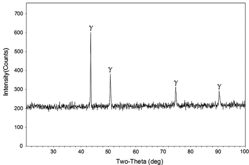
**Fig. 1.** XRD result of the 316LN austenitic stainless steel.
