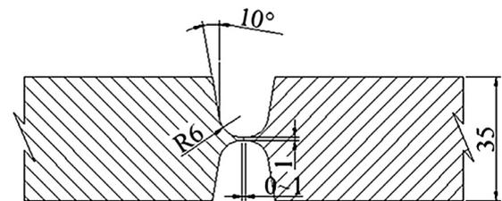
**Fig. 2.** Groove design of welding joint.
