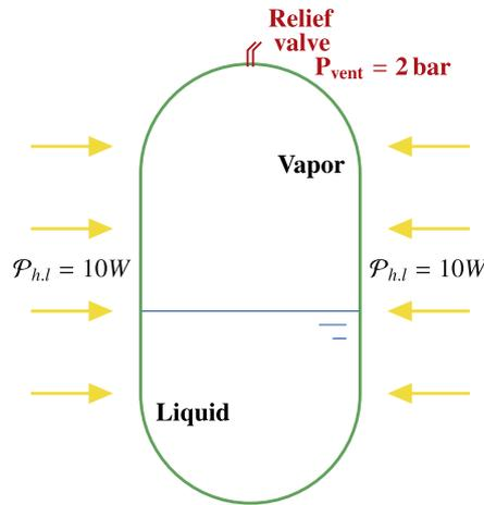
Fig. 1. Schematic view of a  $LH_2$  tank submitted to a 10 W heat load and regulated thanks to a relief valve triggered at 2 bar.
