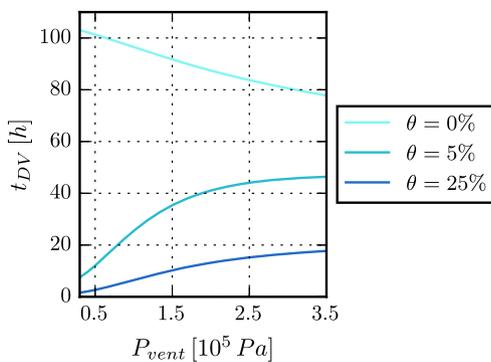
Fig. 3. Influence of the relief valve venting pressure ( $p_{vent}$ ) and the liquid mass fraction of the expelled propellant ( $\theta$ ) on the DV venting time for a 137 L tank submitted to 10 W heat load.
