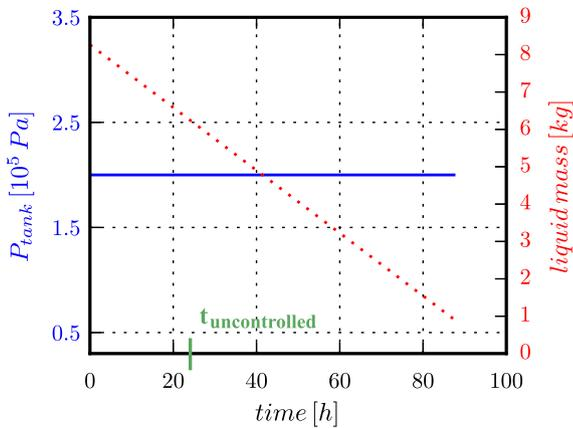
Fig. 2. Pressure (blue) and liquid mass (red) evolution in 137 L tank initially filled at 90% during a DV pressure regulation. The un-controlled tank life expectancy is specified by the green dash. (For interpretation of the references to color in this figure legend, the reader is referred to the web version of this article.)
