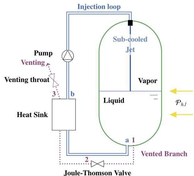
Fig. 4. Schematic view of a TVS controlled tank. The (blue) injection loop drives directly a subcooled jet inside the ullage. The (violet) vented branch creates the cold source heat sink. (For interpretation of the references to color in this figure legend, the reader is referred to the web version of this article.)
