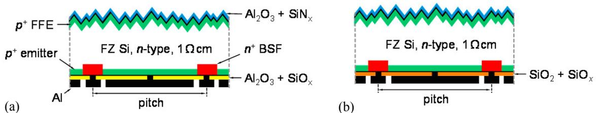
Fig. 1. Schematic of the IBC solar cells with BSF formed by local ion implantation of phosphorus and subsequent  $BBr_3$  furnace diffusion to form the emitter and anneal the phosphorus implantation [7]. The pitch is 0.5 mm with 0.4 mm emitter width and 0.1 mm BSF width. The cells were processed identically, but the thermally grown  $SiO_2$  was either kept as back-side passivation layer and capped with  $SiO_x$  (b) or replaced by an  $Al_2O_3 / SiO_x$  stack (a). (FFE = front floating emitter)
