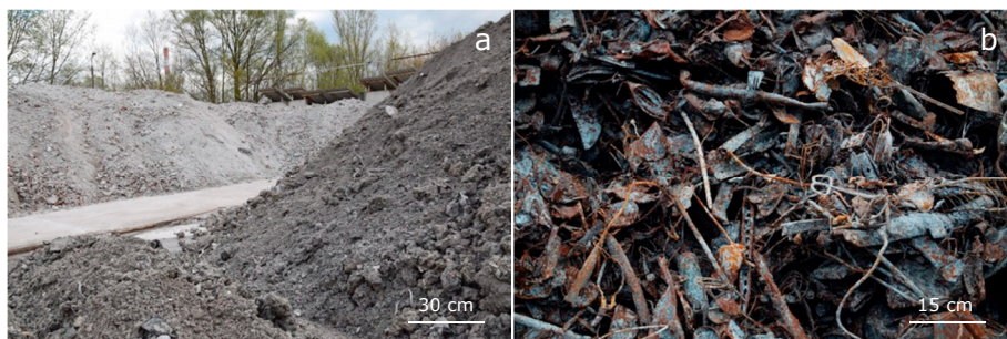
Fig. 1. (a) fresh BA stored on a heap; (b) metallic products separated from the BA using hand picking and magnetic separator.
