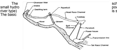
schematic of a power plant (run-ofis shown in Fig. 1. Download English Version:
