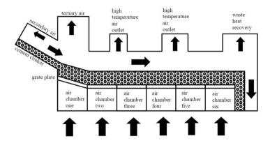
Fig. 1. the cooling process of the grate cooler
