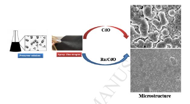
Preparation of undoped and Ru doped CdO thin films and surface microstructure of deposited CdO thin films.
