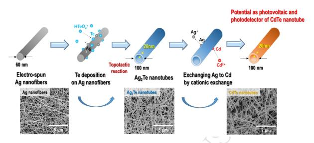
High throughput synthesis of CdTe nanotubes by combinational process
