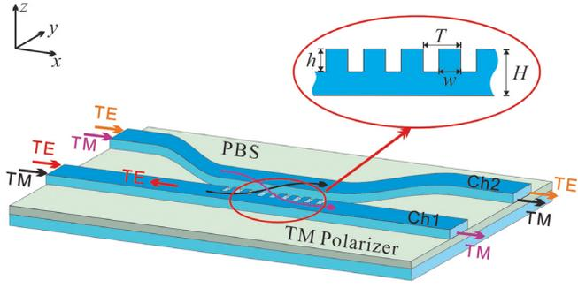
Fig. 1. The structure of TM-mode-pass polarizer and polarization beam splitter, which consists of two channels named as Ch1 and Ch2, respectively.
