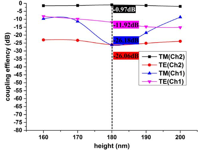
Fig. 2. The coupling efficiency of different polarization in two channels versus the etch height, which has an optimized value of 180 nm.
