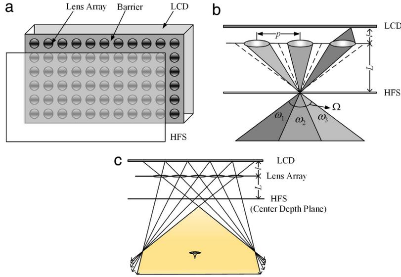
Fig. 1. (a) The structure of the LFD, (b) the diffuse of the HFS, (c) the viewing zone of the display.
