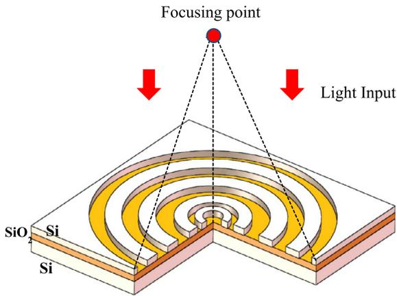
Fig. 1. Schematic representation of the CC-HCG reflector.
