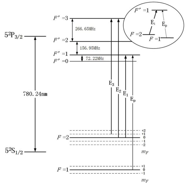
Fig. 2. The relevant energy levels of  $D_2$  transition of  $^{87}\text{Rb}$  for our experiment. Inset, three-level  $A$ -type system.
