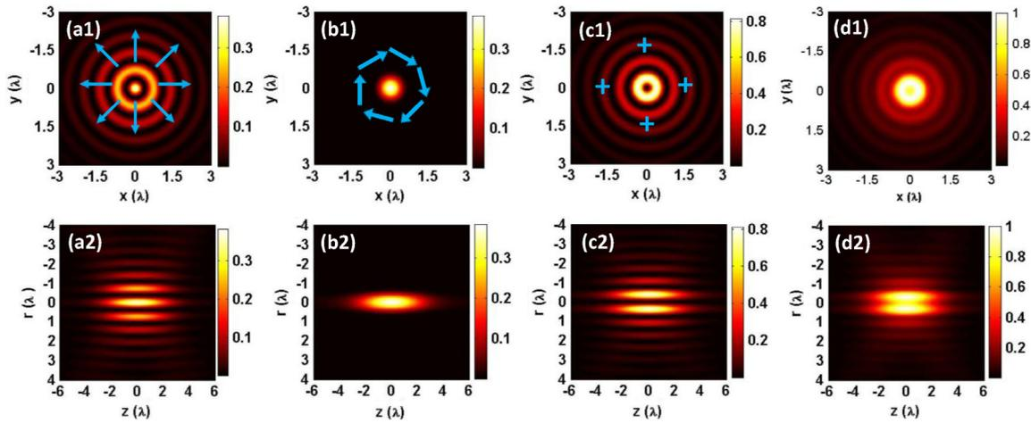
**Fig. 1.** Tight focusing behaviors of radially polarized CAVB in the focal plane under the conditions of  $a = 0.05$ ,  $r_c = 1$  mm,  $l = 1$ ,  $\lambda = 633$  nm,  $w = 0.08$  mm,  $NA = 0.85$ ,  $f = 1$  mm. Top panels (a1–d1) and bottom panels (a2–d2) are the radial, azimuthal, longitudinal components and total intensity patterns in  $x$ - $y$  and  $r$ - $z$  plane, respectively.
