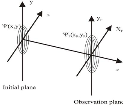
Fig. 1. Propagation of a field from an initial plane with coordinates  $(x, y)$  up to an observation plane with coordinates  $(x_F, y_F)$ . The planes are parallel to each other and separated a distance  $z$ . The amplitude distributions are  $\Psi(x, y)$  and  $\Psi_F(x_F, y_F)$  respectively.
