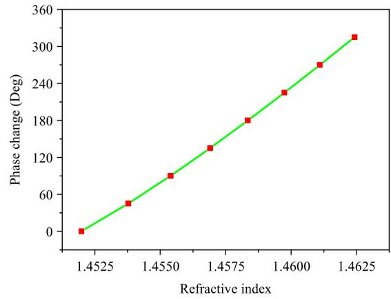
Fig. 2. Phase change as a function of the core refractive index. Solid green curve corresponds to theoretical predictions using Eq. (2), square red dots are the designed phase change points.
