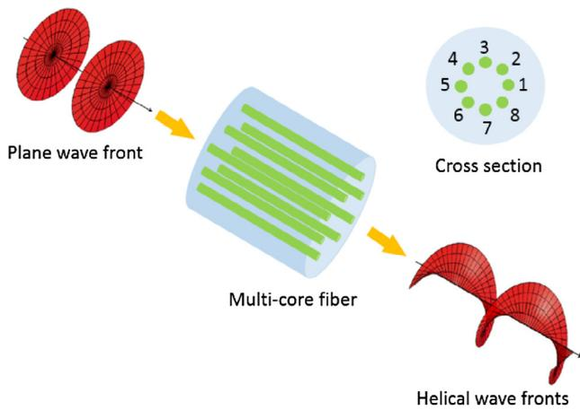
Fig. 1. Schematic of a multi-core optical fiber that induces wavefront shaping.
