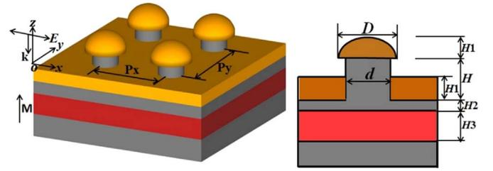
Fig. 1. A schematic of the tri-layer structure under consideration on a glass substrate: the right subplot is the cross-section in the  $x$ - $z$  plane. The structure is illuminated by normally TM-polarized light that has the electric field parallel to  $x$  axis.
