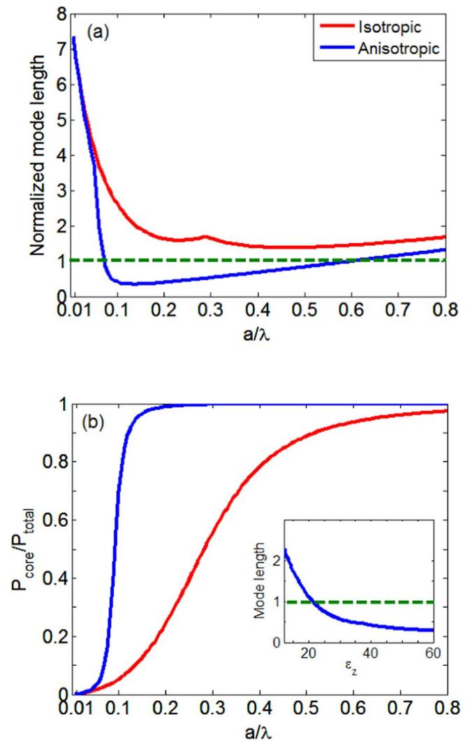
**Fig. 3.** Mode length comparison of slab waveguides with the core size. It shows that the anisotropic core ( $\epsilon_x = 2.6, \epsilon_z = 40$ ) can grasp TM mode to subdiffraction values. Inset: the total power completely concentrates in the core across a large range of the core size as compared to the case in conventional waveguide.
