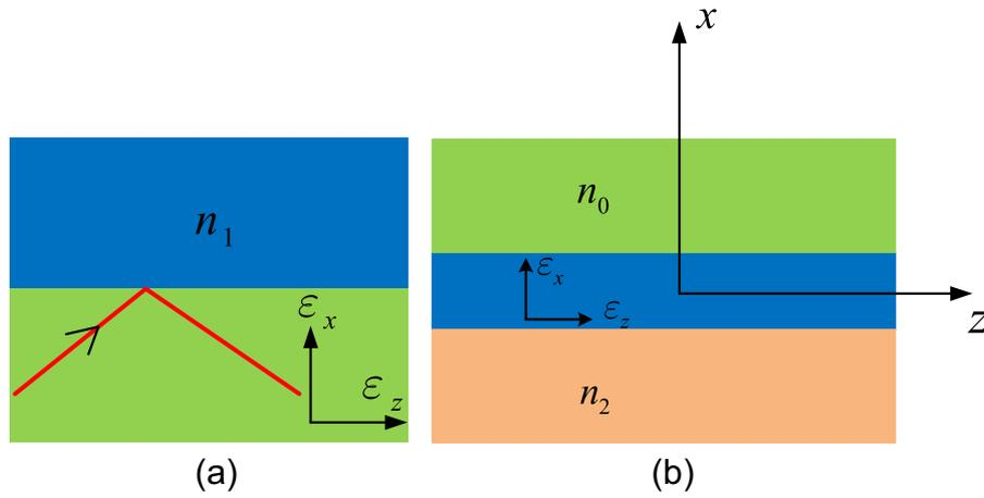
**Fig. 1.** (a) Relaxed-TIR: the condition for TIR is relaxed to  $\sqrt{\epsilon_x} > n_1$  when light moves from anisotropic medium ( $\epsilon_x, \epsilon_z$ ) to dielectric  $n_1$ ; (b) slab waveguide based on Relaxed-TIR:  $\sqrt{\epsilon_x} > n_0$  and  $\sqrt{\epsilon_x} > n_2$  preserve the conventional waveguiding mechanism, the wave can be confined inside the core using anisotropy ( $\epsilon_z \gg 1$ ).
