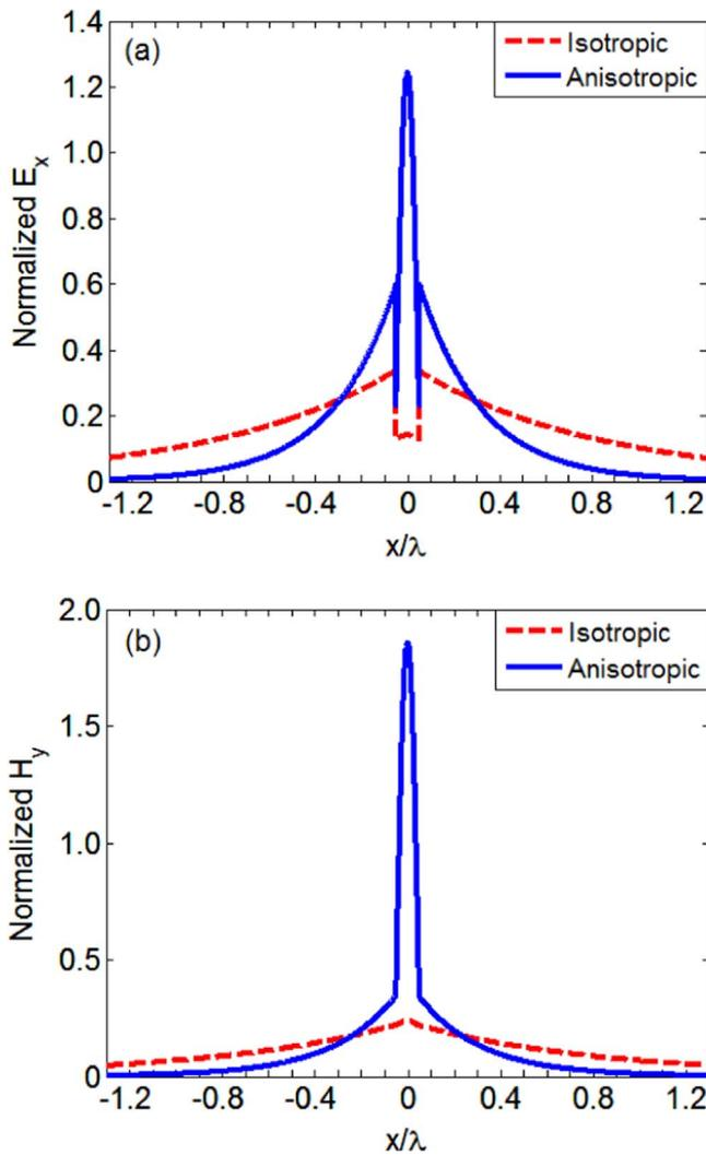
**Fig. 2.** Normalized (a)  $E_x$  and (b)  $H_y$  profiles of TM mode for a slab waveguide with all-dielectric metamaterial core ( $\epsilon_x = 2.6, \epsilon_z = 40$ ) surrounded by air (solid line) on comparison to the case of a conventional waveguide ( $\epsilon_x = \epsilon_z = 2.6$ ) (dashed line). The core size is  $0.1 \lambda$ . Inset: the mode length achieves subdiffraction deeply as  $\epsilon_z$  increases.
