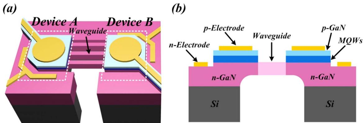
Fig. 1. A schematic of the device structure: (a) top view; (b) side view.
