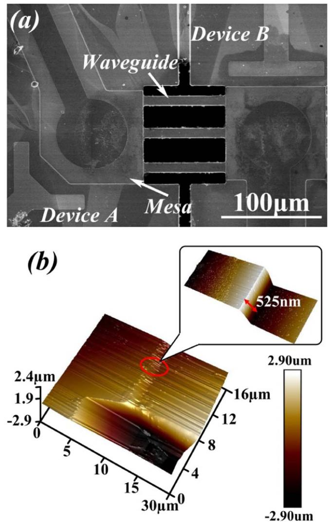
Fig. 2. (a) SEM image of the fabricated in-plane VLC system, (b) an AFM image of the suspended waveguide.
