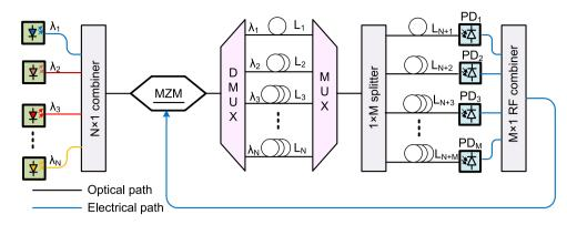
Fig. 1. Conceptual diagram of WDM multi-loop OEO. MZM:Mach-Zehnder modulator, DMUX:Demultiplexer, MUX:Multiplexer, PD:photodiode.
