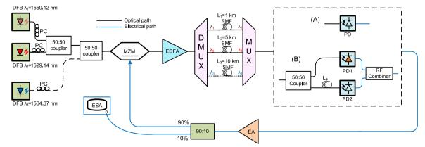
Fig. 2. Schematic diagram of the experimental WDM multi loop OEO based on either two or three laser sources and one photodiode (A) or two photodiodes (B). PC:Polarization Controller, DMUX:Demultiplexer, MUX:Multiplexer, SMF:Single Mode Fiber, ESA:Electrical Spectrum Analyzer.
