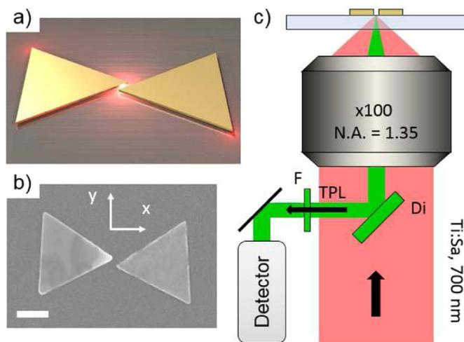
**Fig. 1.** (a) Artistic view of a multimodal bowtie antenna composed of two prismatic plasmonic cavities. (b) SEM image of a symmetric bowtie antenna made of two pristine colloidal gold prisms. scale bar represents 200 nm. (c) Schematic drawing of our home made microscope in which a femtosecond laser beam tuned at  $\lambda_L = 700$  nm has been used for the experiments.
