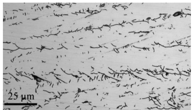
Fig. 2. Surface crack in silicon wafer sliced by fixed diamond wire saw (Würzner et al., 2015).
