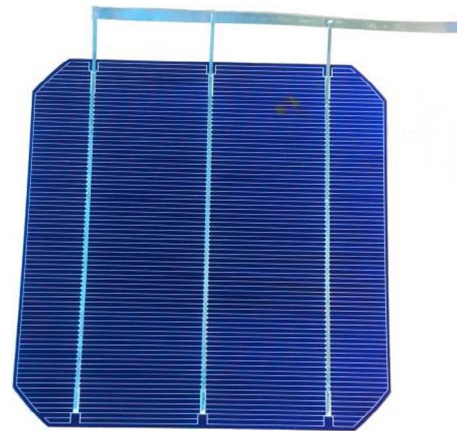
Fig. 1. Image of specimen (soldered monocrystalline silicon solar cell).
