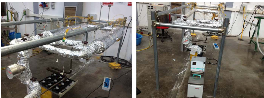
Fig. 1. Storage elements of SolTeCa1 experimental plant.
