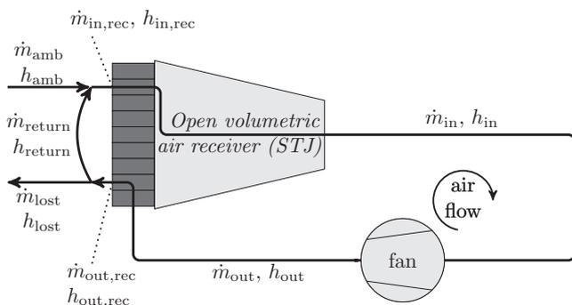
**Fig. 2.** A schematic of the open volumetric receiver is shown. The air mass flows  $\dot{m}$  and specific enthalpies  $h$  are indicated.
